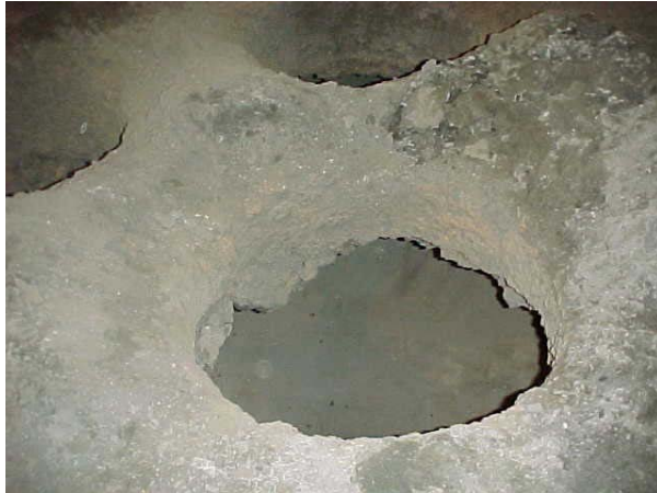
Fig. 6: Precast delta with high emissivity coating after approximately 2/3 of its service life. The delta was put back into service, where it provided over 100 additional heats.
